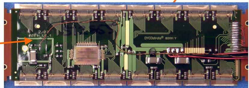
Detection of charged particles takes place in 1744 identical *ATLAS Pixel Modules*
