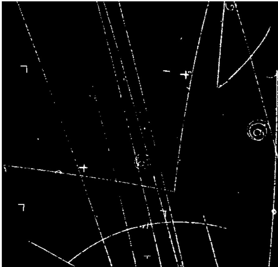
“Tracks” of ionized particles due to charged particles traversing a “bubble chamber”—one kind of particle detector.
